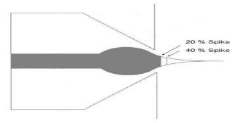
Figure 2: Truncated Plug Nozzle 20% and 40%
