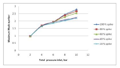
Figure 9: Maximum Mach Number in the Flow Domain for Various Total Pressure Inlets
