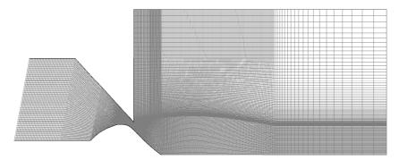
Figure 6: Grid System for Full Spike (100%) Nozzle
