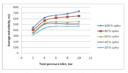
Figure 10: Average Exit Velocity in the Flow Domain for Various Total Pressure Inlets
