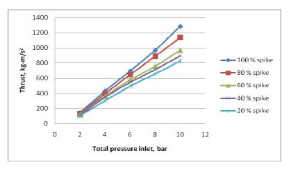
Figure 11: Thrust Produced for Various Total Pressure Inlets
