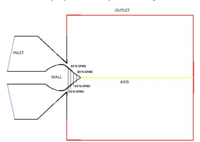
Figure 4: Geometry of Aeropsike Nozzle Configuration
