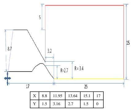
Figure 5: Geometry Model Used for without Trucation
