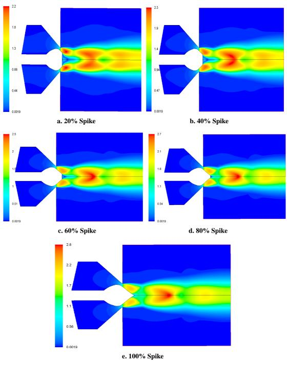
Figure 8: Mach Number Contours in Different Spike Configurations for a Total Pressure Inlet 10 Bar
